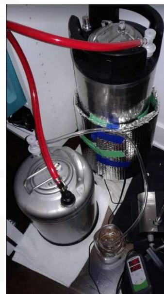
I ferment in kegs, so prefer using a heat-wrap and a temp controller.
